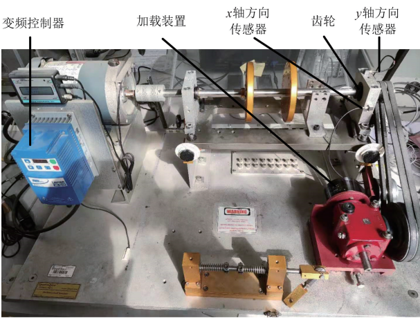
图 14 滚轴齿轮故障模拟实验平台 Fig. 14 Experimental platform for simulation of roller gear failure
