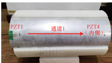
图 11 管道多通道通信实验 Fig. 11 Schematic diagram of multichannel communication experiment in pipelines
