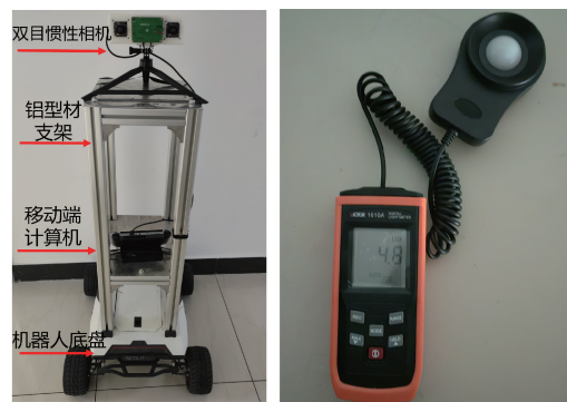
(a) 图像采集设备 (b) 数字光照度计 (a) Image acquisition equipment (b) Digital illuminometer
