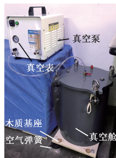
(c) 矢量传感器本底噪声测试平台 (c) Vector sensor noise floor measurement platform
