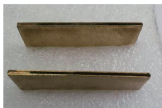
(a) 弯曲层合梁结构 [121]
