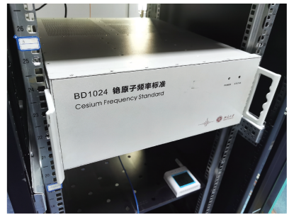
(a) BD1024的4U整机实拍 (a) Picture of the 4U size prototype BD1024
