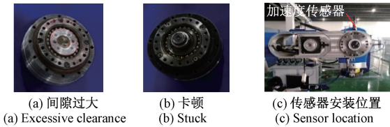
图3 谐波减速器状态及传感器安装位置 Fig. 3 Harmonic reducer status and sensor location
