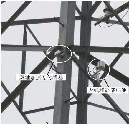
(b) 双轴加速度传感器安装图 (b) Installation diagram of biaxial acceleration sensor
