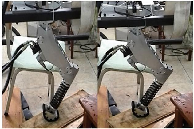
(e) 开始触地阶段 (e) Start touch down stage (f) 屈膝压缩阶段 (f) Knee compression stage
