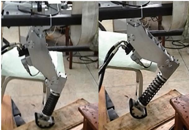
(a) 起跳初始阶段 (a) Take-off initial stage (b) 腾空阶段 (b) Flight stage
