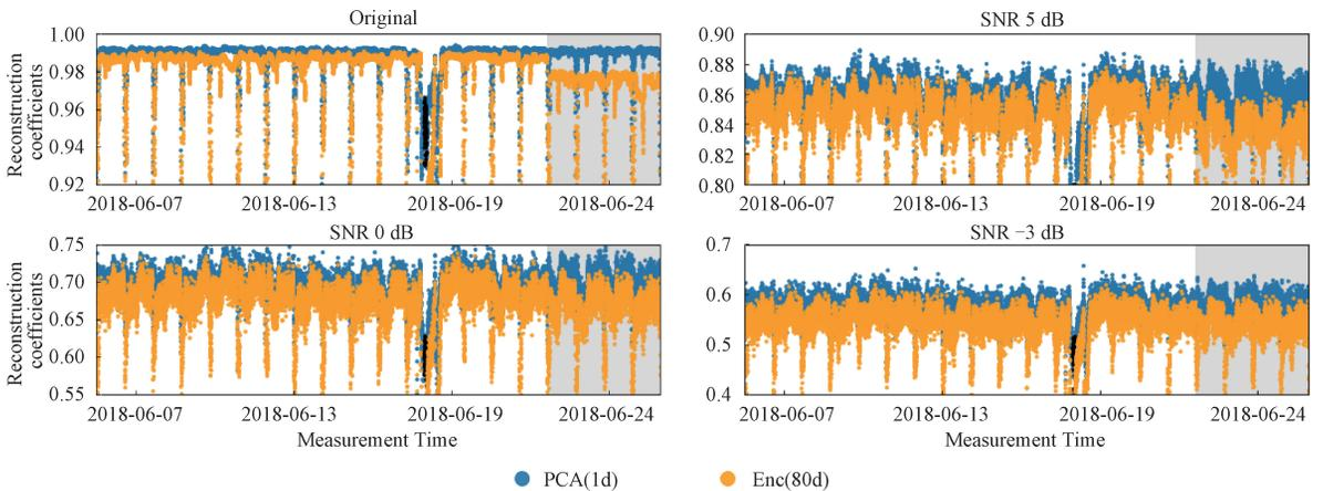
Fig. 2 The reconstruction coefficients of guided waves by short-term PCA and autoencoder with varying signal-to-noise ratios (噪声环境中自编码神经网络重建系数变化图)
