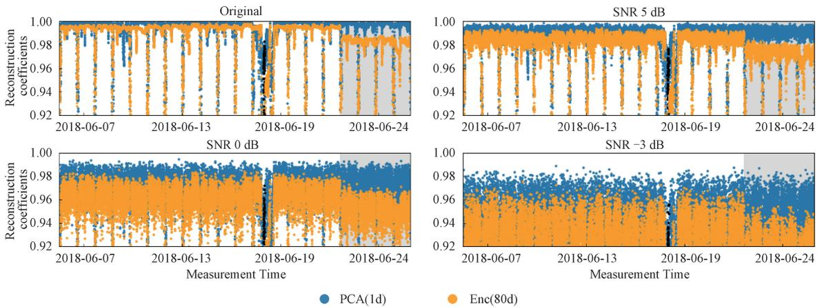
Fig. 3 The reconstruction coefficients of guided waves by PCA and autoencoder with varying signal-to noise ratios after using denoised (应用降噪算法后, 噪声环境中自编码神经网络重建系数变化图)
