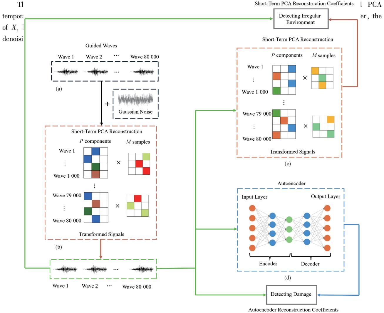
Fig. 1 The damage detection framework incorporating a denoising module is depicted (噪声环境中故障检测算法框架图):
