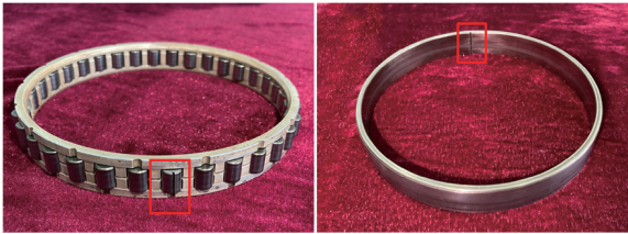
图 6 中介轴承滚动体和外圈故障示意图 Fig. 6 Diagram of roller and outer ring failures in intermediary bearing
