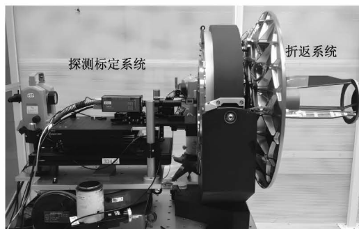
图6 RTA 单星点激光目标模拟系统 Fig. 6 Single star point laser target simulation system of RTA
