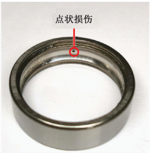
图 10 故障轴承外圈 Fig. 10 Outer ring of fault bearing
