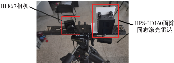
图6 相机和激光雷达的位置关系 Fig. 6 Positional relationship between camera and lidar
