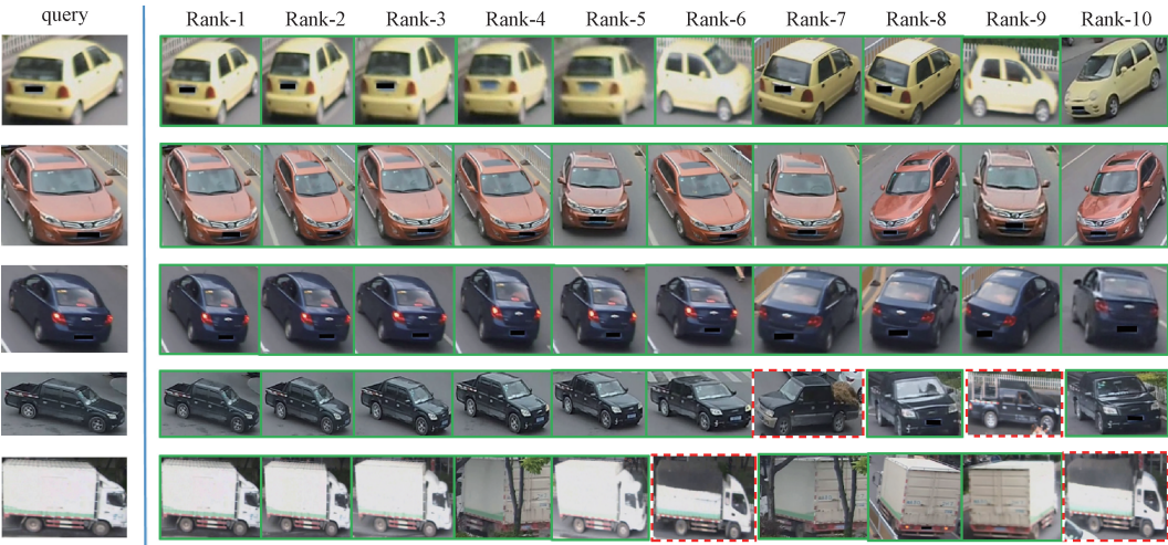
图 4 车辆重识别结果 Fig. 4 Results of vehicle re-identification
