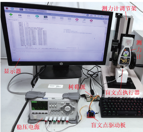
图 9 测试盲文点执行器上弹力与锁止力的实验平台 Fig. 9 Experimental platform for testing upper elastic force and locking force of Braille dot actuators
