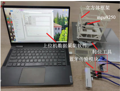
图 5 实验装置与数据采集 Fig. 5 Experimental equipment and data acquisition
