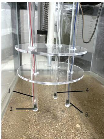
1-发射电极正极;2-接收电极正极;3-接收电极负极;4-发射电极负极
