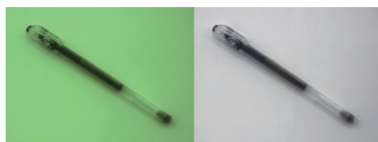
(a) 白平衡调节前 (a) Before white balance adjustment (b) 白平衡调节后 (b) After white balance adjustment
