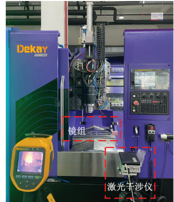
(a) 测试现场 (a) The test site
