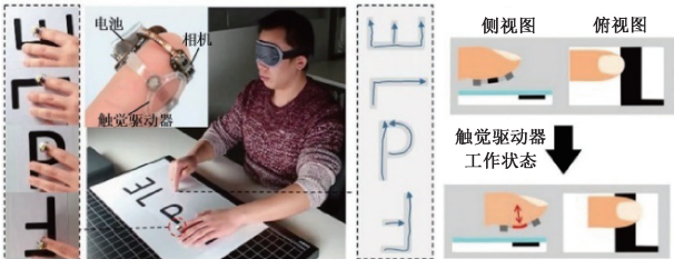
(e) 帮助视障用户通过手指“看见”文字的触觉反馈设备 (e) A haptic feedback device helps visually impaired users "see" text with their fingers
