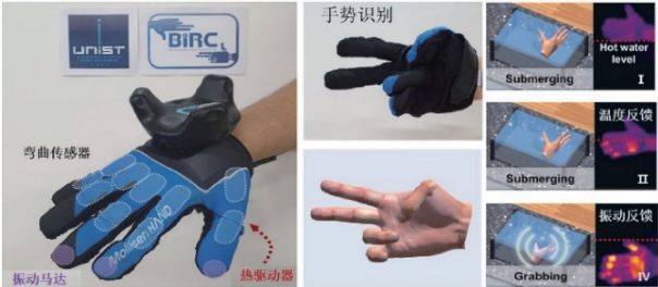
(a) 用于VR中温度反馈的触觉反馈手套 (a) A haptic feedback glove for thermal sensation in VR
