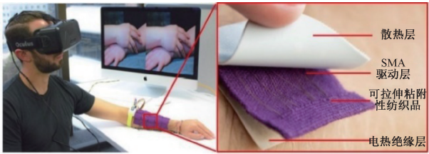
(a) 基于SMA的贴片式触觉反馈驱动器 (a) SMA based plasters for haptic feedback
