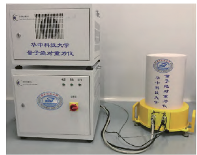
(a) 车载原子干涉重力仪MAIN (a) The vehicle-mounted atomic interference gravimeter MAIN
