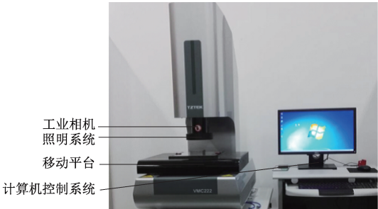
图 3 图像采集平台 Fig.3 Image acquisition platform
