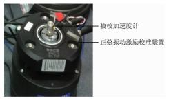
正弦振动激励校准装置 Fig. 8 The device of calibration upon sinusoidal excitation
