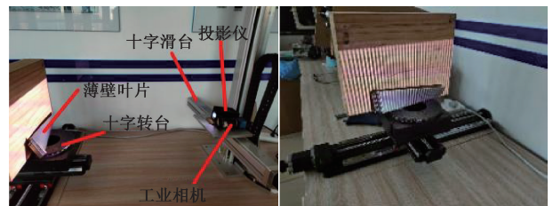
(a) 整体实验平台 (a) Overall test platform (b) 点云数据采集 (b) Point cloud data acquisition
