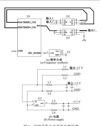
图 3 双频采集合成系统电路原理 Fig. 3 Circuit schematic of the dual-frequency acquisition synthesis system
