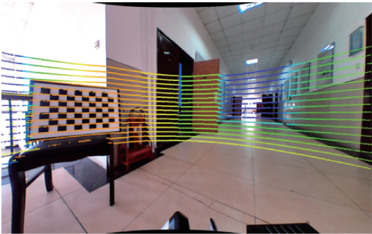
(b) 点云投影 (按距离可视化) (b) Point cloud projection (visualization per distances)
