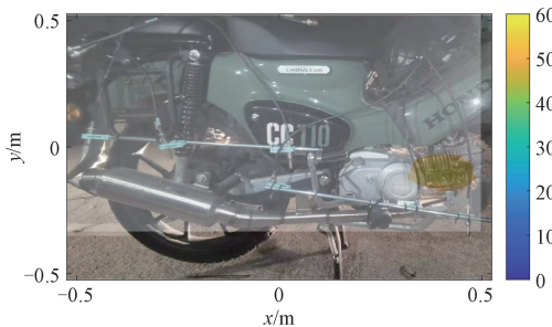
图 9 情形一下基于 TLS 的频率为 700 Hz 处的声全息图 Fig. 9 Acoustic hologram based on TLS obtained at the frequency 700 Hz for first operating condition
